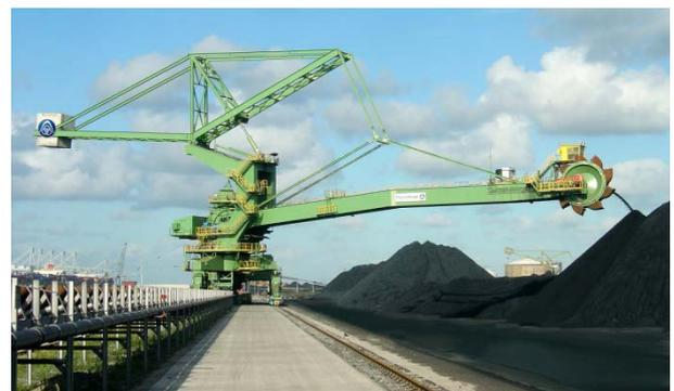
Figure 2: Bucket wheel stacker/reclaimer (Courtesy of ThyssenKrupp)
