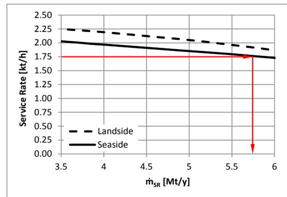
Figure 8: Service rates versus the stacker/reclaimer annual throughput for the FIFO+ operational procedure
