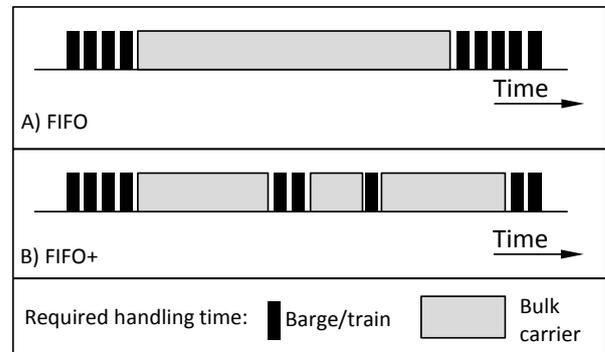
Figure 4: Two different operational procedures
